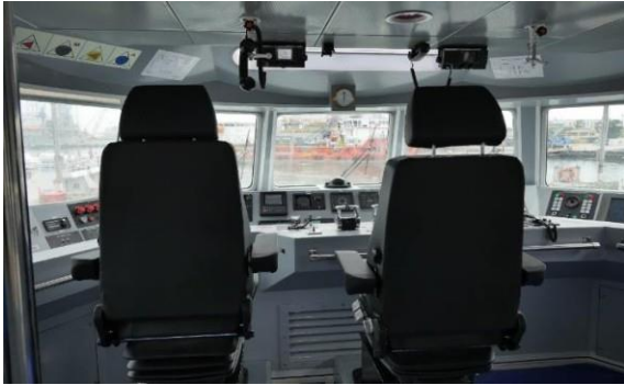
Forward bridge console with all-round view
